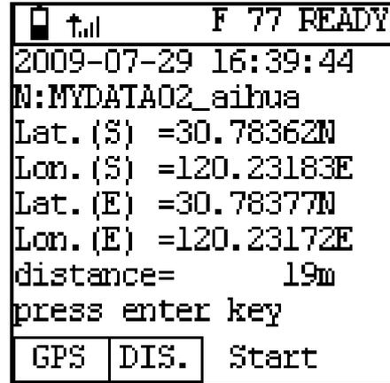
When the meter is moved to the starting point, press the Enter key. After the meter is moved to the ending point, the user can view the coordinates of the two points and their linear distance.
