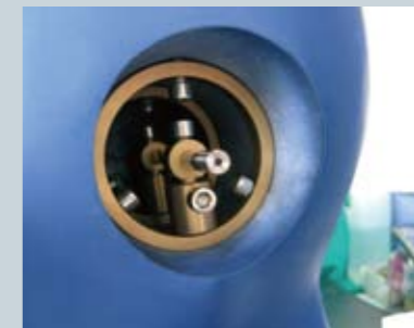
The ear on the artificial head can be removed so that the microphones inside the artificial head can be easily calibrated.
